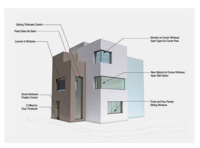
In Vectorworks 2016, improved window and door functions give you more options to create compelling designs. From three- and four-panel sliding windows, to span wall options for corner windows, to control over door hardware positioning,\* designers will be able to add more depth (and more data) to their projects than ever before.
